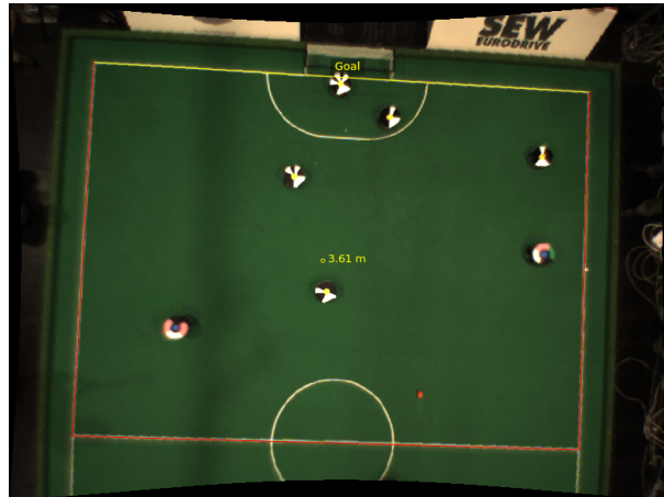
Fig. 7. Distortion corrected camera image with field lines
