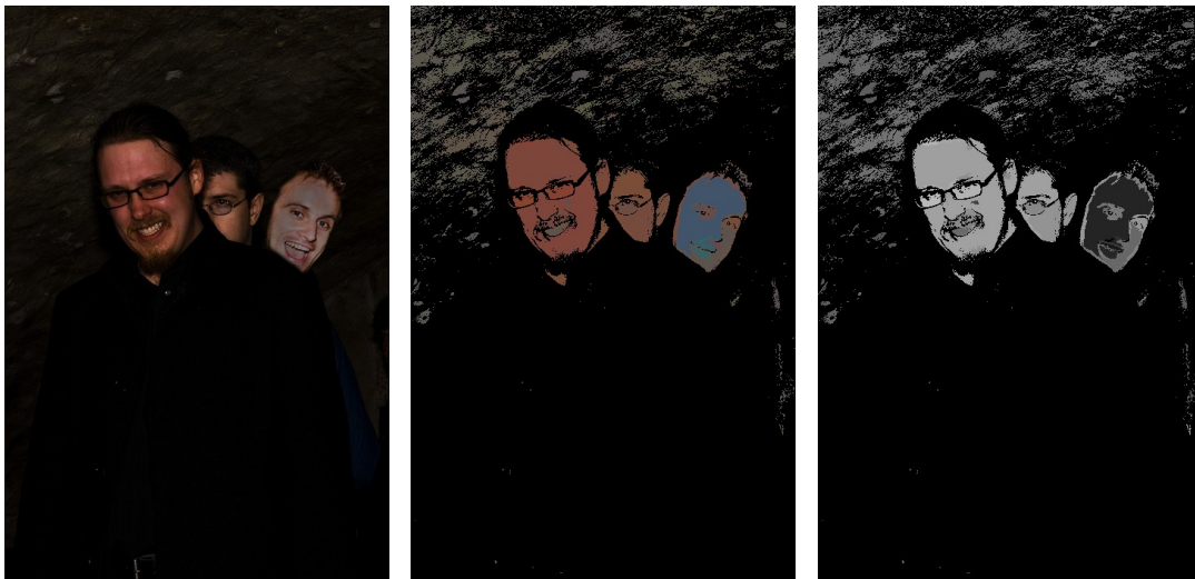
Figure 5.4: Tampered image. Illumination map as well as distance map show a clear difference between the first two and the third person. Since the three stand close together in the image, it can be assumed that this difference is due to tampering.
