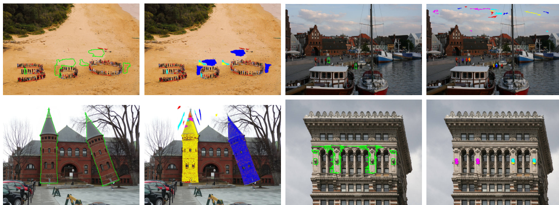
Figure 2.15: Indicative performance of SURF (left) versus ZERNIKE (right) features. Top left: Plain copy-move example, SURF and ZERNIKE detect all copies. Top right: JPEG compression quality of 70 hides the copied people from the SURF keypoints. ZERNIKE generates many false positives in homogeneous regions. Bottom left: 20^\circ rotation of the snippet is easily handled by both, SURF and ZERNIKE. Bottom right: Combined transformations, in addition to highly symmetric image content, result in SURF producing a large number of false positives. The block-based ZERNIKE features correctly detect the copied statues.
