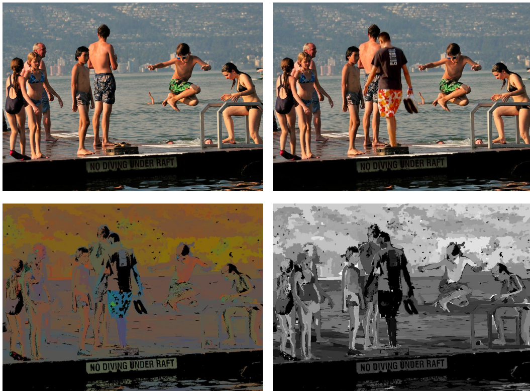
Figure 5.5: Original image (top left) and tampered image (top right). A comparison of the skin regions of the people exposes the inserted man in the distance map.
