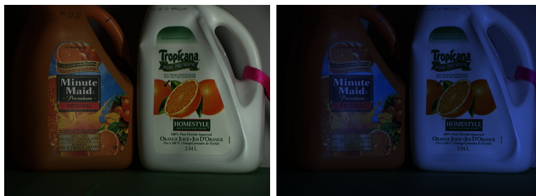
Figure 4.1: Example of the influence of illumination on the perceived object color. The same scene is shown, once exposed to white illumination, once exposed to illuminants that approximate illumination at night. The pictures are part of the dataset by Barnard et al. [Barn02b]).
