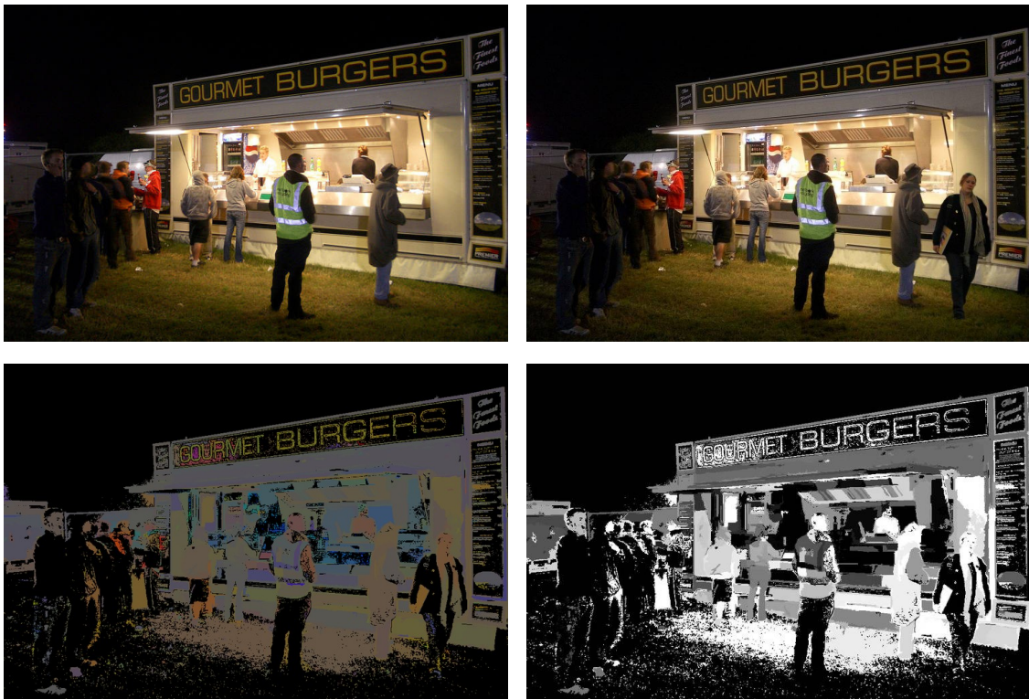
Figure 5.6: Original image (top left) and tampered image (top right). At first glance, illumination map and distance map show plausible results on the tampered image. However, the illuminant estimates are obtained from the front of the inserted woman, which is turned away from the restaurant lights. Therefore, the expected illumination should be more bluish, like e.g. at the back of the person in the middle.
