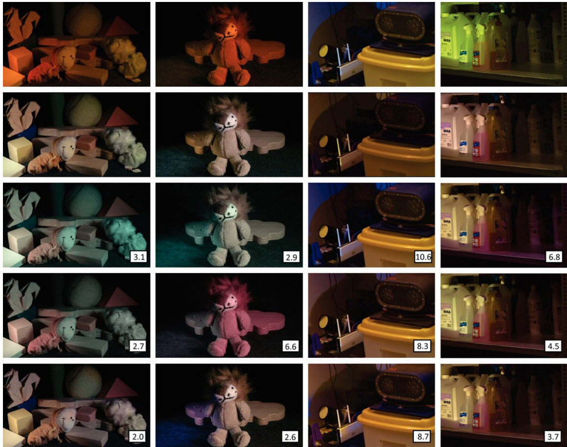
Figure 4.24: Examples for automated white balancing (WB). From top to bottom the rows present: original image from the camera, the WB images using the ground truth, global Gray World, Gijsenij et al. [Gijs12b], and MIRF. Note that the images are enhanced to sRGB for visualization. The captions on the images denote their estimation error.
