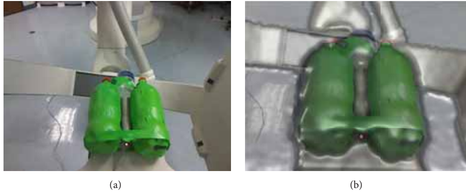
FIGURE 6: (a) shows an RGB image of the knee phantoms acquired by the Kinect camera. The corresponding preprocessed RGBD image can be seen in (b).
