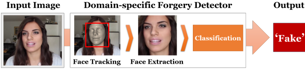
Figure 5: Our domain-specific forgery detection pipeline for facial manipulations: the input image is processed by a robust face tracking method; we use the information to extract the region of the image covered by the face; this region is fed into a learned classification network that outputs the prediction.
