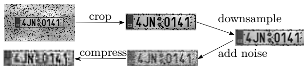
Fig. 2. The pipeline for generating license plates consists of five steps. First, the frame and font are printed and cropped. Then the image is degraded by downsampling, additive noise, and compression.
