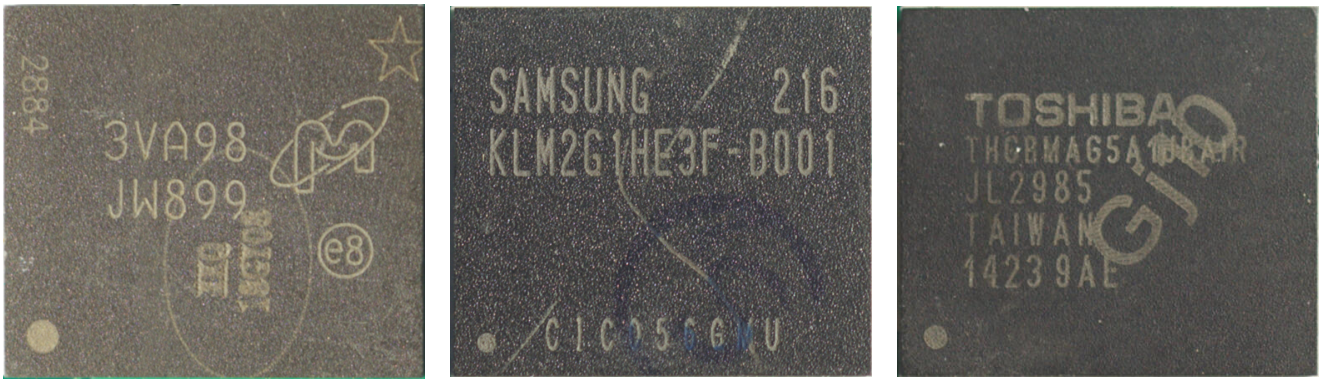
Figure 3: Example NAND chips with irregular stamps on it.
