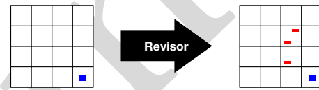
Figure 6: Data view of the revisor, showing the mutated metadata before and the checksum corrected data afterward.
